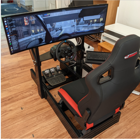
Figure 1: Driving simulator set up using CARLA. A human driver emulates the AV stack for testing and evaluating the proposed data recorder.
