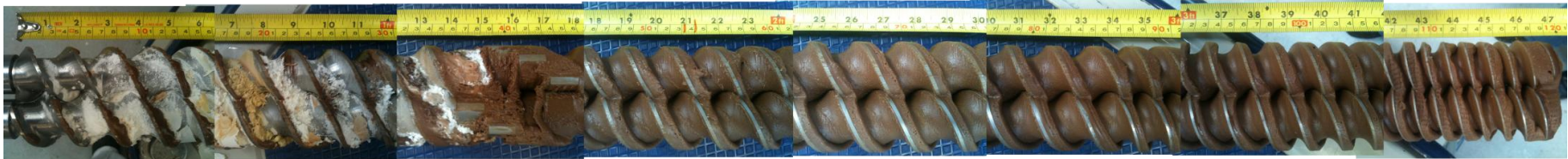
Figure 7.8 Dead-stop screw photo of paste S2 - 100 kg/hr - 300rpm - 8% water - with Mixing Element
