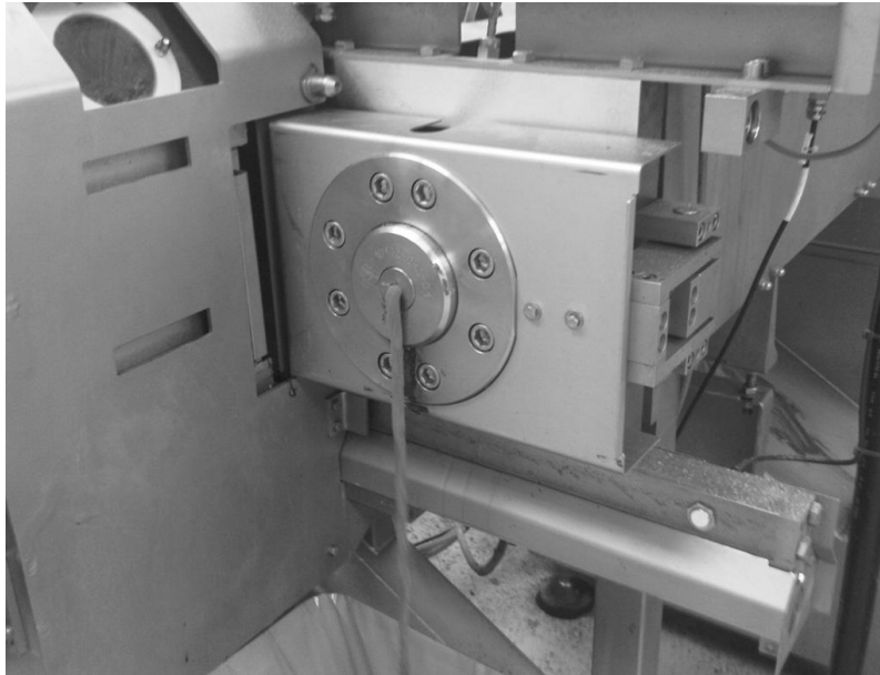
Figure 7.3 Extruder endplate with circular die
