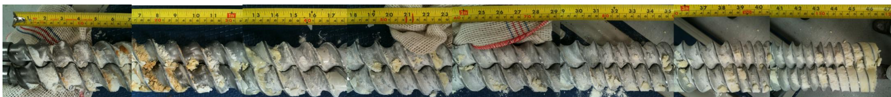
Figure 7.26 Dead-stop screw photo of paste S9 - 100 kg/hr - 300 rpm - 5% water (no CM) - no Mixing Element
