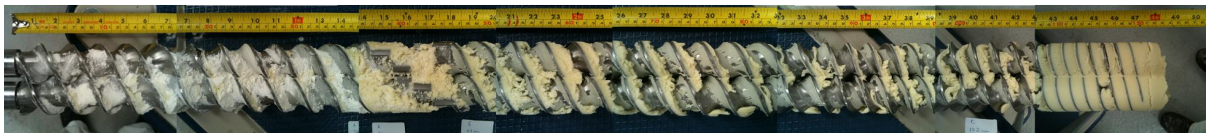
Figure 7.23 Dead-stop screw photo of paste S6 - 100 kg/hr - 300 rpm - 5% water (no CM) - with Mixing Element
