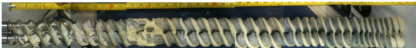
Figure 7.24 Dead-stop screw photo of paste S7 - 100 kg/hr - 300 rpm - 8% water (no CM) - with Mixing Element
