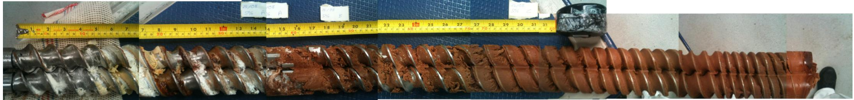
Figure 7.7 Dead-stop screw photo of paste S1 - 100 kg/hr - 300rpm - 5% water - with Mixing Element
