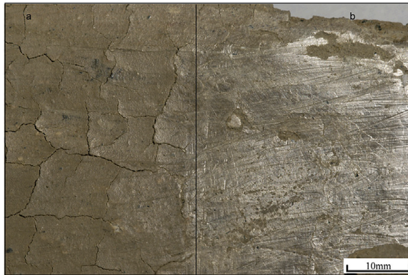
3. 46. (a) Soft leather-hard and (b) stiff leather-hard paste, reproduced from Lepère (2014: 147, Figure 2).
