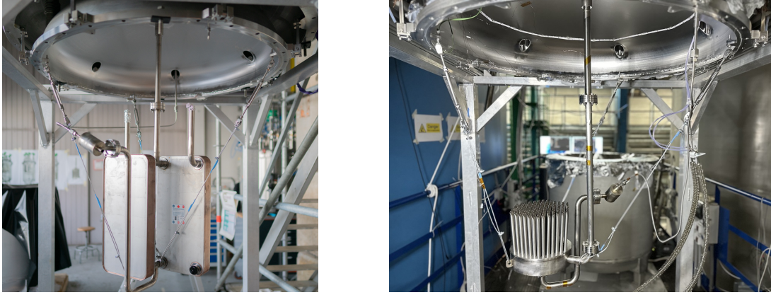
Figure 5. Pictures of the two-phase heat exchangers inside the cryostat. (Left): Parallel plate geometry. (Right): Multi-tube geometry.
