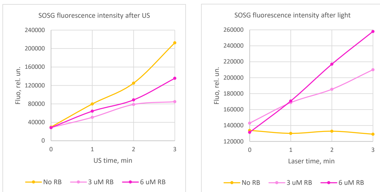
Fig. 5.3.1.4. SOSG fluorescence after a sample with RB was either sonicated or exposed to green light. Samples had 1.5 \mu\text{M} SOSG and varying concentrations of RB; sonicated samples had DBPC-PEG40S MBs ( \sim 5 \times 10^7 MBs/mL), and for ultrasound t = 0 were ruptured manually in a syringe. In this experiment, sonication was performed in an ultrasound bath (150W, 40kHz) in 2 mL plastic tubes, and exposure to light was carried out as described in the Methods section. For the laser measurements, fluorescence gain setting was 1800, and for the sonicated samples it was 1450.
