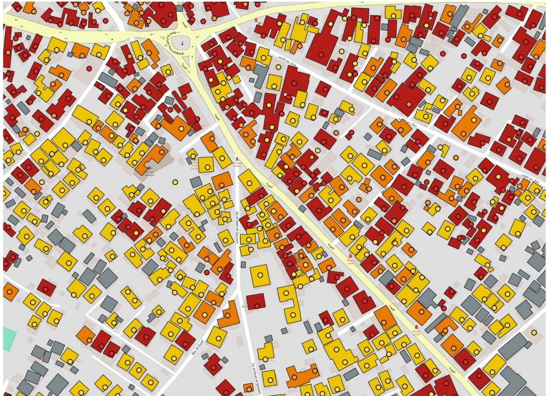
Figure 2. Matching building footprints to nearby damage classifications. Affected footprints inherit the highest damage classification of points within 4 m: moderate damage (yellow), severe damage (orange), and destroyed (red). Footprints for which there are no points within 4 m are assumed to be intact (grey). Map data from © OpenStreetMap contributors.
