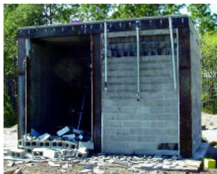
Figure 1.1 Non-coated (left) and rubber coated (right) masonry walls after blast loadings (Porter et al., 2002)
