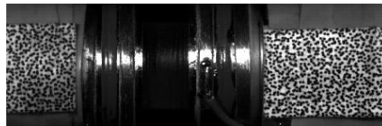
Figure 7.11 High speed imaging on the modified SHPB: the printed speckle pattern is attached on the surface of the bars near the PZT sensors, a silicone rubber specimen sits in the middle.
