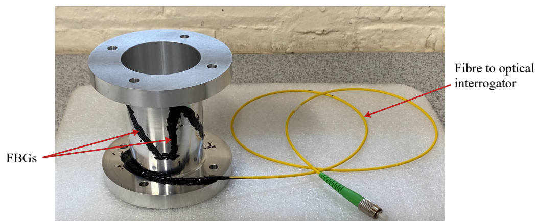
Figure 3.23 Prototype of the exemplar column-type sensor instrumented with eight FBGs using the layout in Figure 3.21
