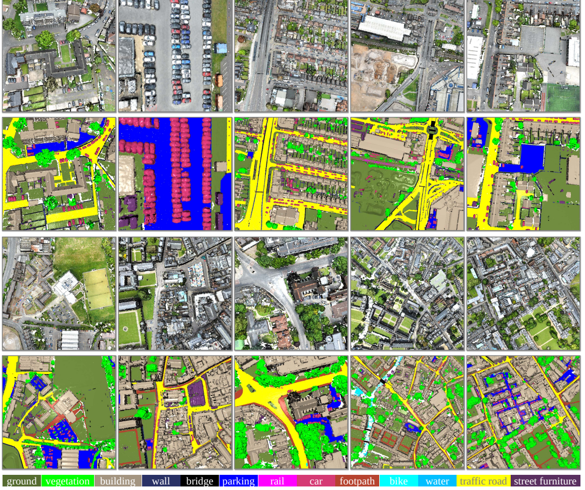
Figure 3.5: Additional examples of our SensatUrban dataset. Different semantic classes are labeled by different colors. The top two rows are point clouds collected from Birmingham, and the bottom two rows are point clouds acquired from Cambridge.
