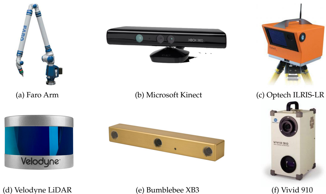
Figure 2.1: An illustration of point cloud acquisition equipment. The source images are adapted from [18, 9, 12, 19, 3, 20].
