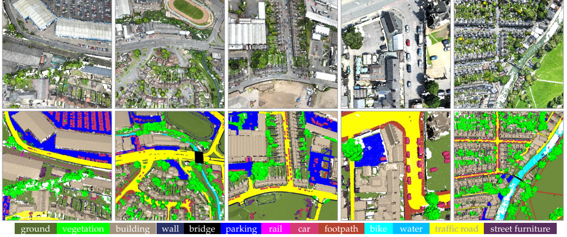
Figure 3.4: Visualization of example point cloud tiles in our SensatUrban dataset. Top: the raw point clouds. Bottom: the semantic annotations of corresponding point clouds. Points belonging to different semantic categories are displayed in different colors.
