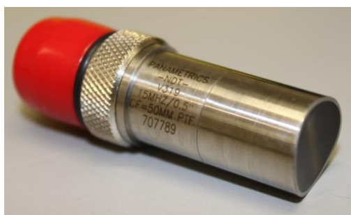
Figure 8-6: Picture of the application specific cylindrical PCD used during all subsequent experiments (left) alongside its frequency response (right). Graph reproduced from the accompanied documentation report, Panametrics-NDT, Olympus.
