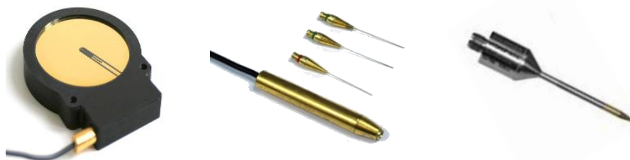
Figure 2-7: A membrane hydrophone (left) and a set of needle hydrophones of different element size each one of which can be screw-connected to the preamplifier base unit (centre). Illustration by courtesy of Precision Acoustics Ltd, Dorchester, Dorset, UK, (left & centre). A robust needle hydrophone that can be inserted in tissue and thus provide in situ pressure measurements (right). Illustration courtesy of ONDA Corporation, Sunnyvale, USA.
