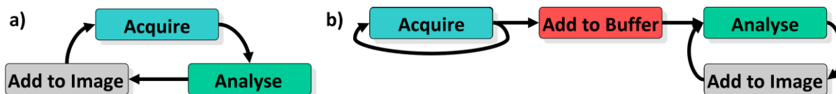
Figure 19 – The schematic difference between performing the centroiding analysis: a) consecutively after image acquisition; b) in parallel.
