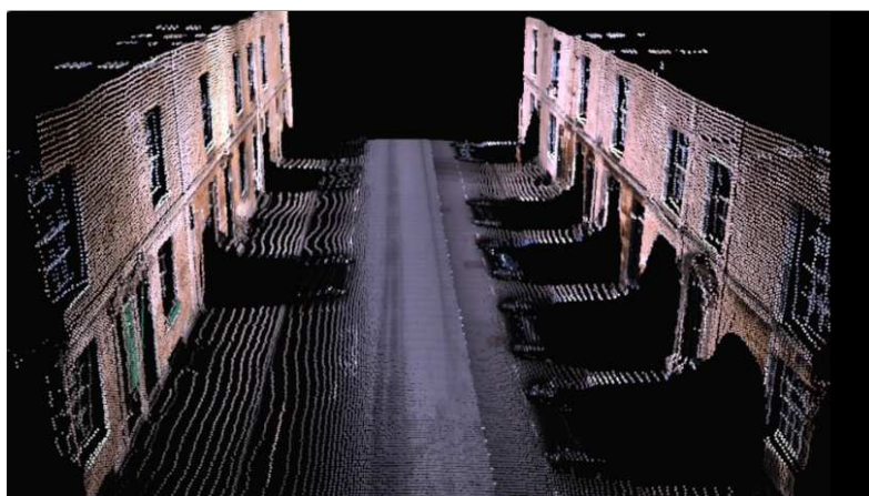
(c) Processed point cloud after automobile removal
