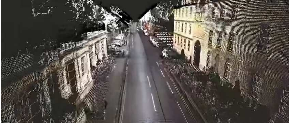
Figure 2.7: Coloured LIDAR Point Cloud Example. Lidar is one of the few sensors on mobile-robotics platforms that provides robust, accurate, and far-ranged depth measurements. The above image plots the lidar point cloud captured by a push-broom LMS-151 (see Figure 2.9 on page 22) in an urban environment. Note how the push broom orientation of the lidar sensor enables it to produce an accurate sparse reconstruction of the 3D structure. Laser points are coloured via cameras that are oriented to provide continuous 360° coverage around the vehicle. Creating sparse reconstructions like this require accurate intrinsic, extrinsic, and temporal calibration [24].
