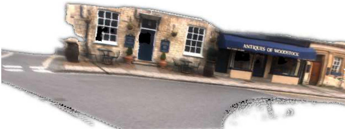
Figure 3.1: An example 3D reconstruction created using the techniques described in this chapter from an automobile’s forward-facing monocular camera.
