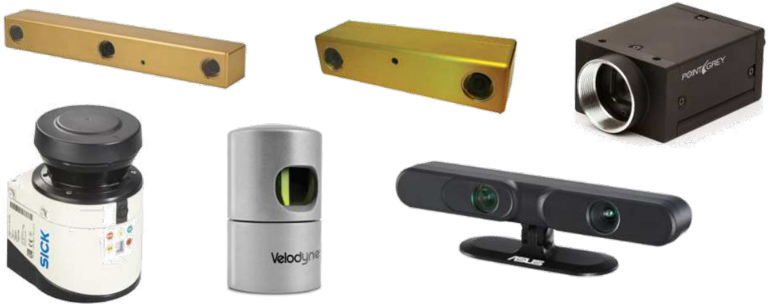
Figure 2.4: Assortment of Sensors. Above are six sensors used in this thesis for dense reconstructions. Clockwise from top-left: (1) Point Grey Bumblebee XB3 colour stereo camera, (2) Point Grey Bumblebee2 colour stereo camera, (3) Point Grey Grasshopper2 colour monocular camera, (4) Asus XtionPro RGB-D camera, (5) Velodyne HDL-32E 3D lidar, and (6) SICK LMS-151 2D lidar. The top row are passive sensors, whereas the bottom row’s sensors actively project light into the environment to measure distances to surfaces.
