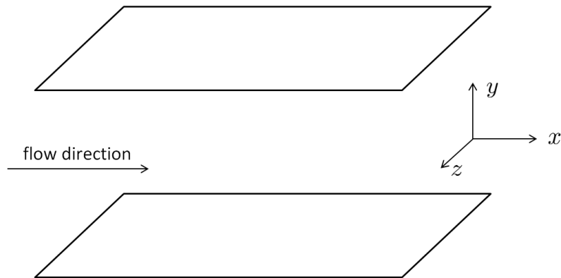
Figure 1.1: Geometry of plane channel flow.
