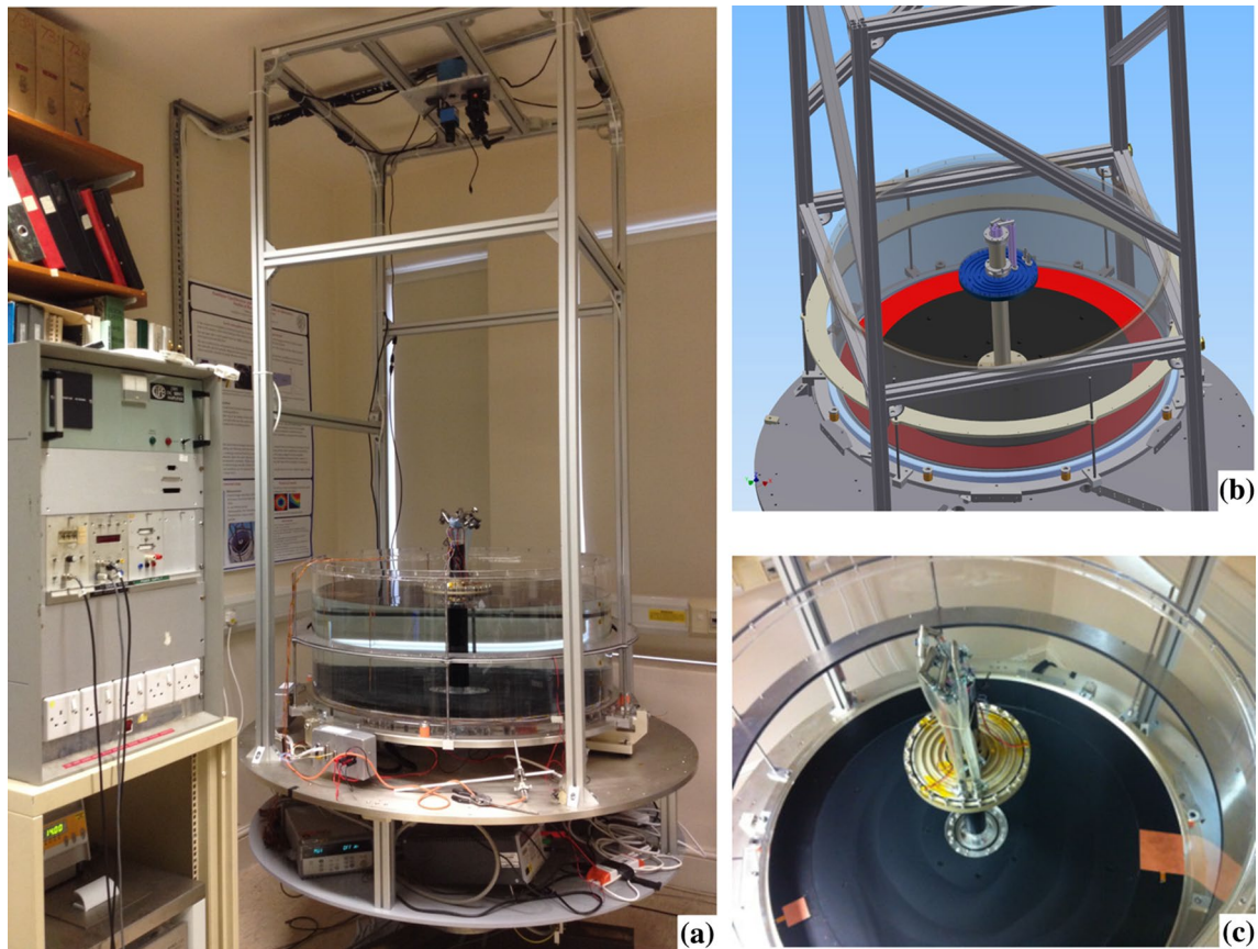
Fig. 3 a Global view of the experimental configuration. The chiller used for the water circulation in the central cold plate can be seen on the left below the turntable control unit in gray . The two vertical rods inside the tank and their corresponding light-brown electrical wires connected to the ten thermocouples can be distinguished on the left-hand side of the tank. b 3D zoomed view of the design of the new setup with the electrically heated annular ring at the bottom of the
