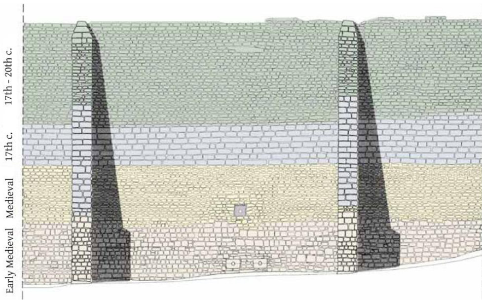
Fig. 3.37 – Mérida: Reconstruction of the constructive phases of the Proserpina dam, labelled in English with Santiago Feijoo’s proposed dating (Feijoo Martínez 2006: fig. 17).
