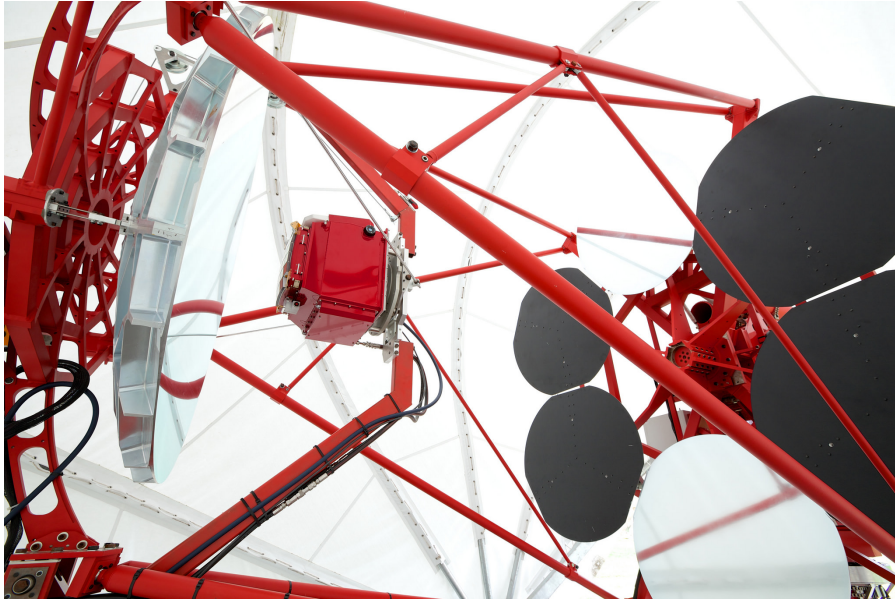
Figure 8.1: Photo of CHEC-M installed on the GCT telescope structure, taken during the first on-telescope campaign [84].
