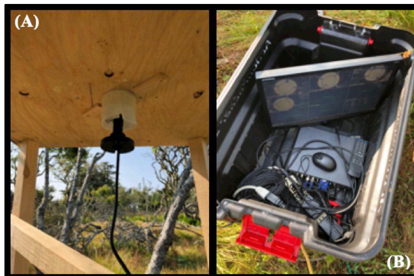
Figure 2.4. Recording setup for orientation cages. (A) CCTV cameras were placed at the bottom of the cage during testing, and videos were recorded onto a DVR. Cameras were positioned so the top of the video pointed towards true North. (B) The monitor and DVR were kept inside of a watertight plastic bin near the cages.
