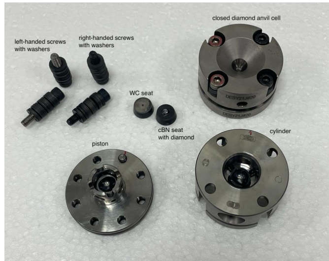
Figure A.1: A short symmetric DAC (right) and a standard symmetric DAC (left) in the opened piston-and-cylinder configuration. Although the closed cell (right) is shorter, both have the same basic setup.
