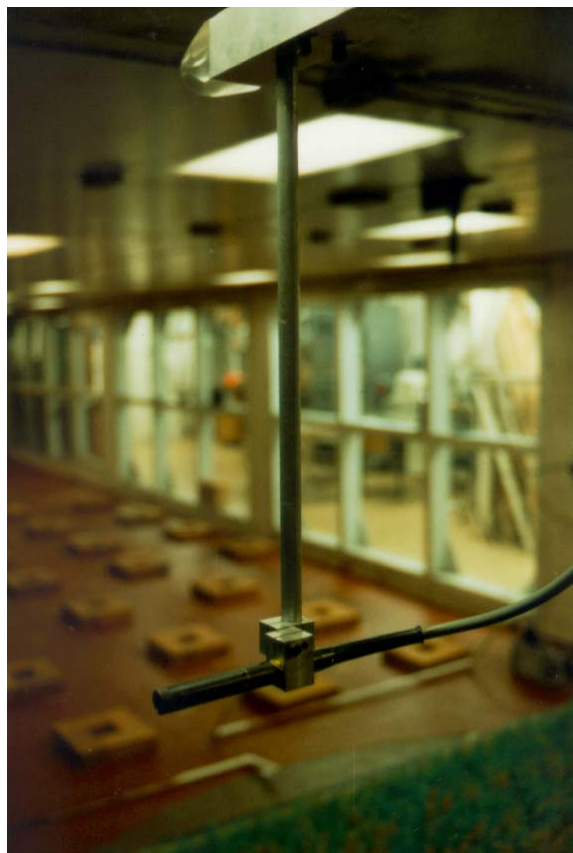
Figure 2.4 LDA probe and support.
