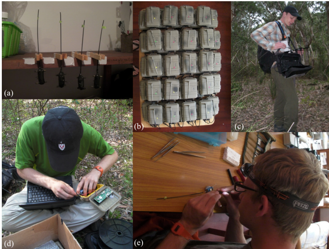
Figure 1. Equipment used to map social networks in wild New Caledonian crows. (a) Tags drying after electronic parts were placed into a protective coating; (b) basestations ready for deployment; (c) Yaggi antenna connected to the computer through a program called pimaster ; (d) basestations being prepared for deployment throughout the study system; (e) tags being prepared for deployment on our study subjects. Photos taken by study team.
