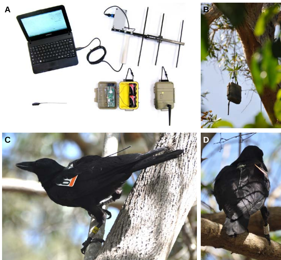
Figure S2, related to Figure 1. Wireless digital transceiver system for the automated mapping of social networks in wild birds ('Encounternet').
