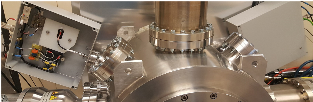
Figure 7.16: Chopper switch boxes attached to VESPA vacuum vessel. Positive box (left) is open to show internal circuitry, including the Behlke switch.
