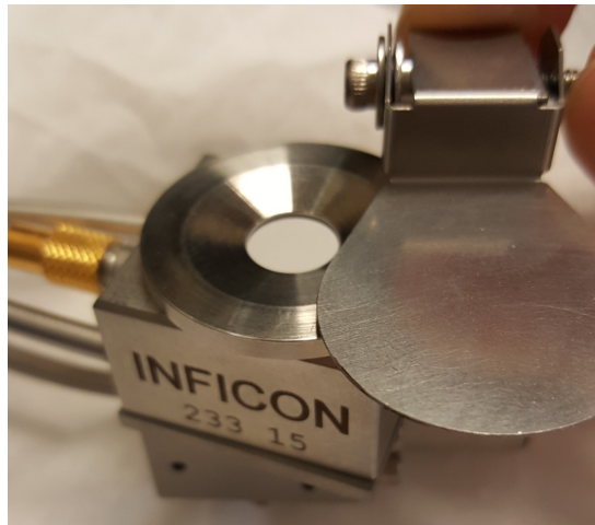
Figure 8.2: Quartz crystal microbalance sensor head with the shutter open.
