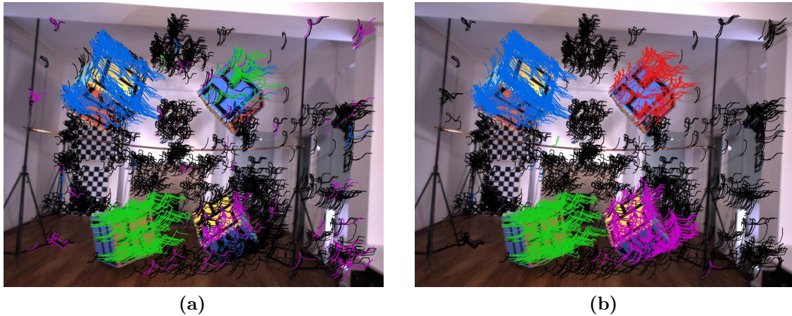
Figure 4.6: A comparison of the segmentations found by a sequential RANSAC (a) and MVO (b) in a single frame of the swinging_4_unconstrained segment of the OMD. Sequential RANSAC not only struggles to find the correct number of models in complex dynamic scenes, but also finds incorrect and oversegmented models.
