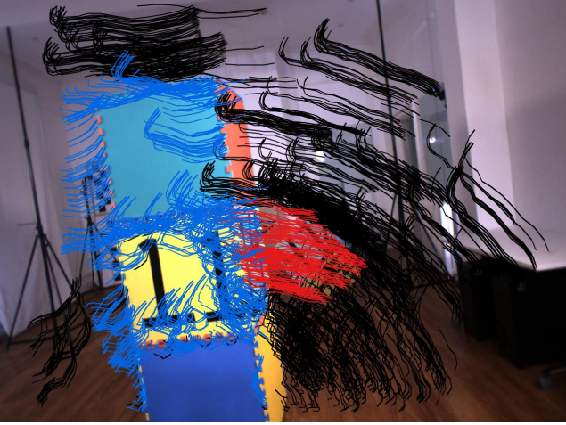
Fig. 4. Motion segmentation produced by occlusion-robust MVO. The egomotion of the camera is estimated from the static points in the scene shown in black. The motions of the swinging block (4, red) and the block tower (1, blue) are segmented and estimated simultaneously with the egomotion.
