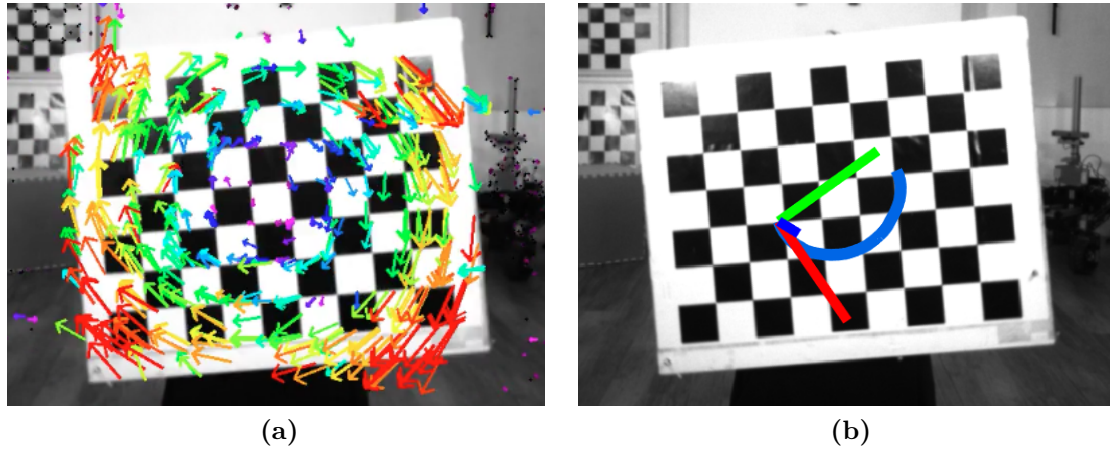
Figure 4.3: Scene flow, (a), and MVO, (b), motion estimation in the pinwheel_1_static segment of the OMD, consisting of a checkerboard rotating about the optical axis of the camera. The magnitude of the flow vector is illustrated by its length and color. Flow techniques inherently calculate individual translational velocities. Since each point on a rotating body has a different tangential velocity, flow techniques fail to segment the velocities into bulk motions. MVO estimates motions as SE(3) transforms even in the presence of rotation. To estimate these motions, flow techniques must solve an equivalent segmentation and estimation problem in the space of velocities.
