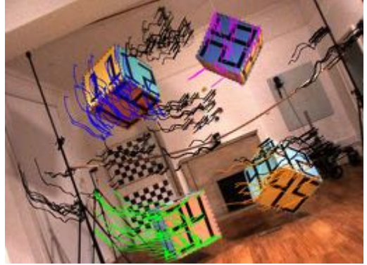
Fig. 1. Motion segmentation produced by our multimotion visual odometry (MVO) system. The egomotion of the camera is estimated from the static points in the scene shown in black. The other colors represent the segmentation of the other motions in the scene.
