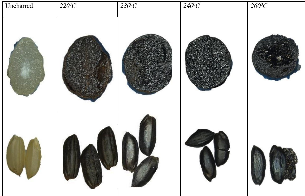
Figure 6. Low power microscopy of modern japonica rice grain heated between 220°C to 260°C (cross-section x2.00 Mag. in the top row and whole-body grain x0.57 Mag. in the bottom row).
