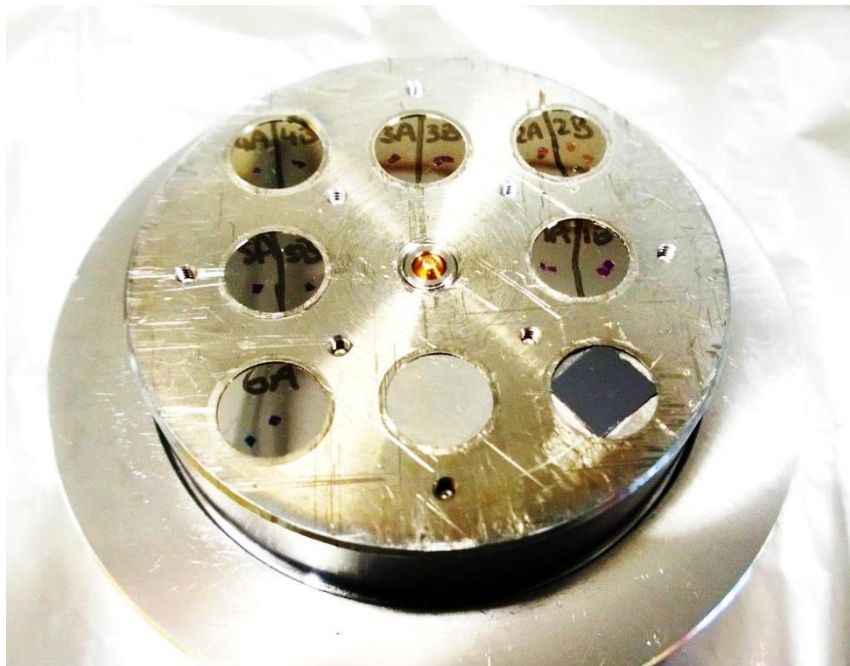
Figure 3.8: Biology sample holder from CAMECA mounted with samples on coverslips and silicon substrates.
