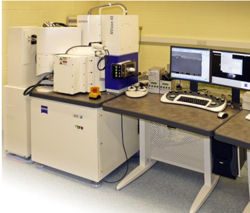
Figure 3.5: The Carl Zeiss NVision dual beam microscope I used for high resolution BSE imaging. From reference [138].
