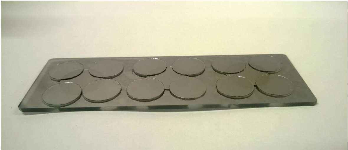
Figure 3.2: Thermanox plastic NanoSIMS substrates for resin section samples, coated with 15 nm platinum on the surface.
