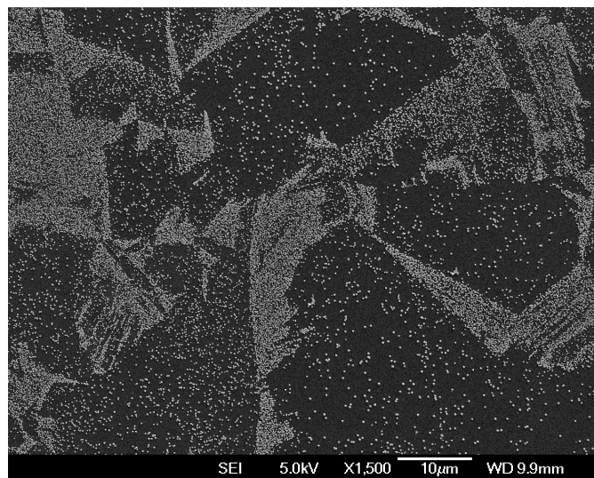
Figure 1.10: SEM image of a nickel modified boron doped diamond electrode, showing the different electroactive domains
