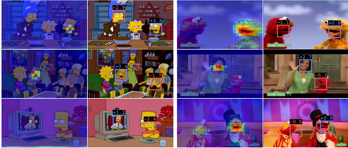
Figure 8.8: Active speaker detection for non-human speakers. We show the top 2 highest-scoring audio-visual objects in each scene, along with the aggregated attention map. Please see our webpage for video results.
