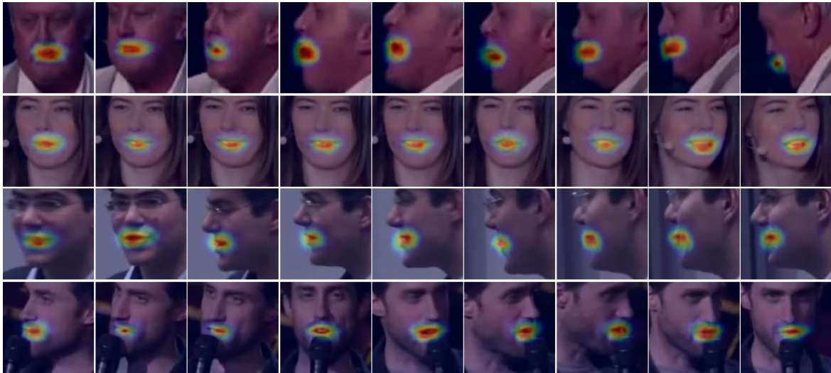
Figure 3.2: Visualization of the visual attention masks \alpha from the VTP module superimposed on the input frames that produce them. The video clips used here are random samples from the LRS3 dataset. It is evident that the model follows the more discriminative mouth region.
