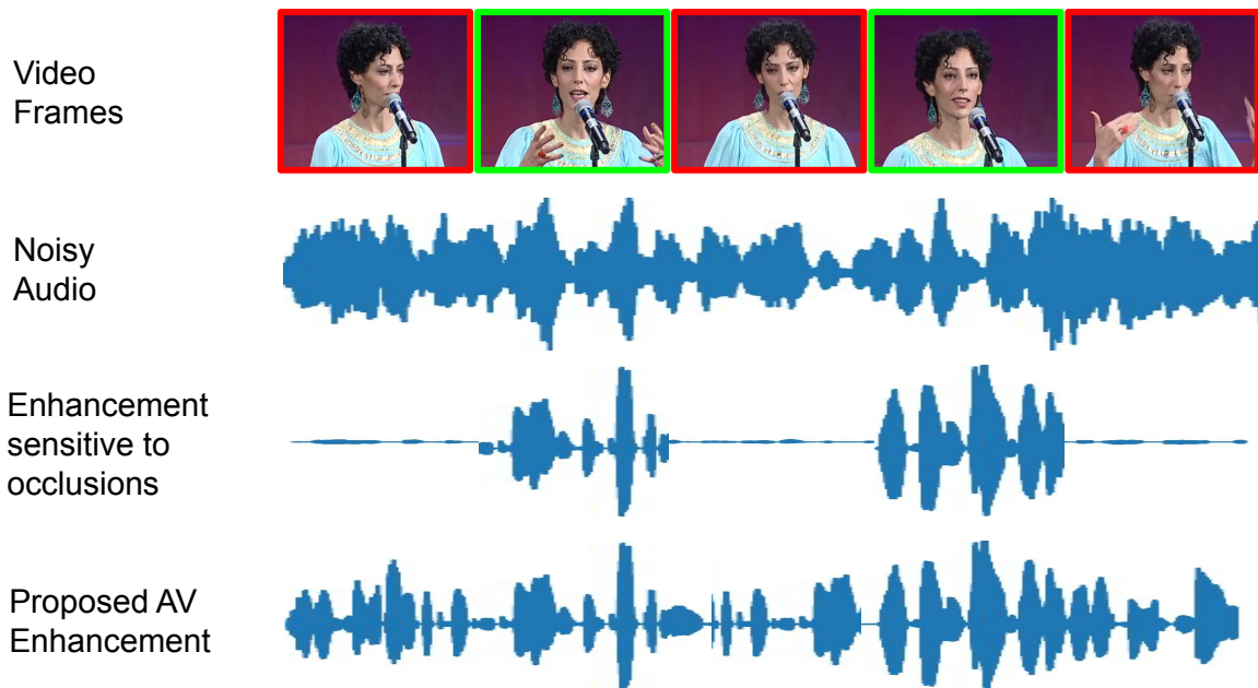
Figure 7.1: An audio-visual speech enhancement model may fail when the lip region is occluded by e.g. a microphone. In such cases the input audio is often entirely filtered out and the result is silent output over the occluded frames. The aim of our method is to be robust to this kind of occlusions.
