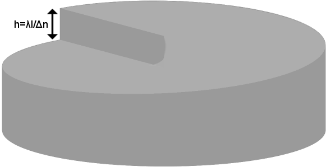
Figure 4.7: Model of a typical transmissive spiral phase plate optimized for converting an input Gaussian to the LG_0^l mode.
