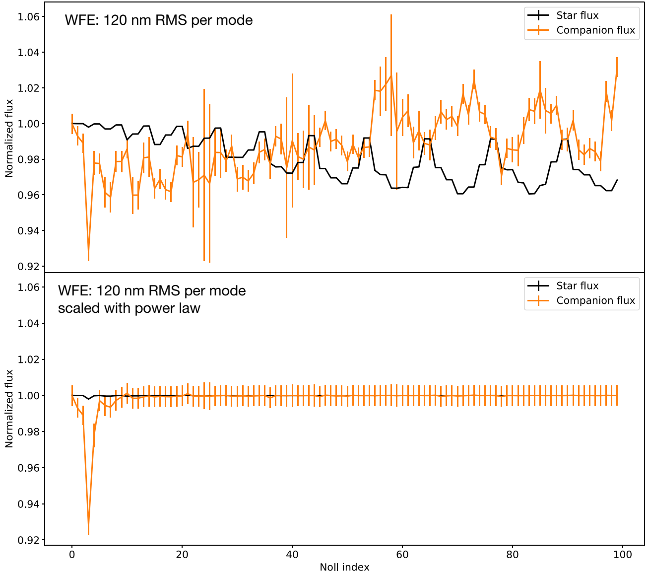
Figure 4. Simulated normalized flux of the star (black) and the companion (orange with visible error bars) for the first 100 Zernike modes, given by their Noll indices. The errors bars indicate the maximum and minimum retrieved companion flux over the observing sequence. The error bars for the star are too small to be visible. Top panel: all Zernike modes have the same 120 nm RMS wavefront error. Bottom panel: the power in the modes is scaled by a power law with a slope of -1.5 , similar to expected NCPAs. In this more realistic scenario, we find that only the lowest order aberrations are likely to significantly impact the average flux of the companion over the observing sequence.
