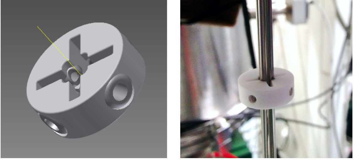
Figure 2.9: The new smaller Macor insulator designed for use in the \varnothing = 35 mm tube of the reducer piece. The left image shows a CAD drawing of the insulator and the right image is a photo of the insulator after installation.
