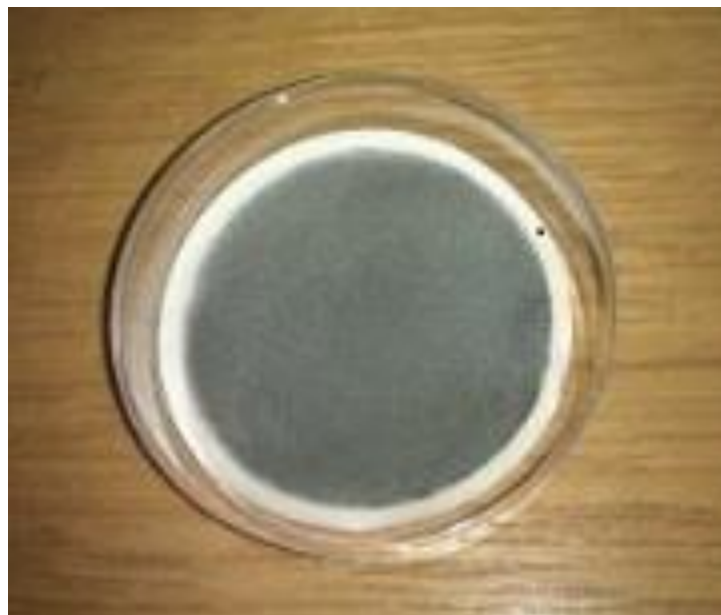
Fig. 3.8 Extracted intermetallic particles on a PTFE filter paper
