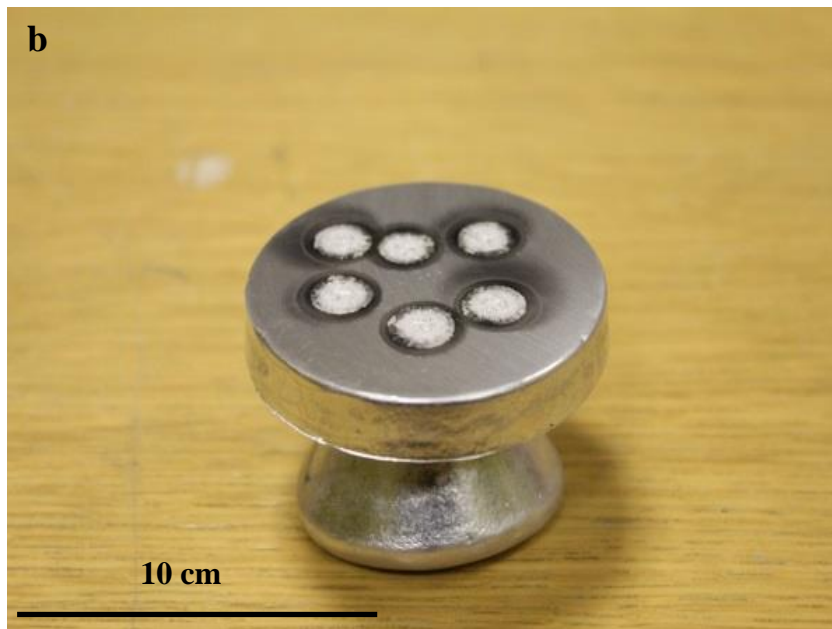
Fig. 3.3 a) Mushroom mould and b) mushroom cast with sparks from OES
