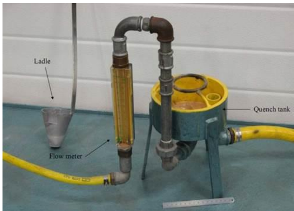
Fig. 3.1 TP1 setup showing different components of the equipment
