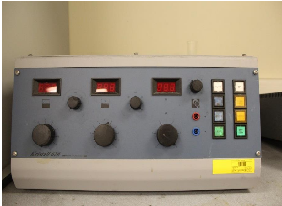
Fig. 3.5 Shows Kristall 620 machine which was used to pass current for anodising.
