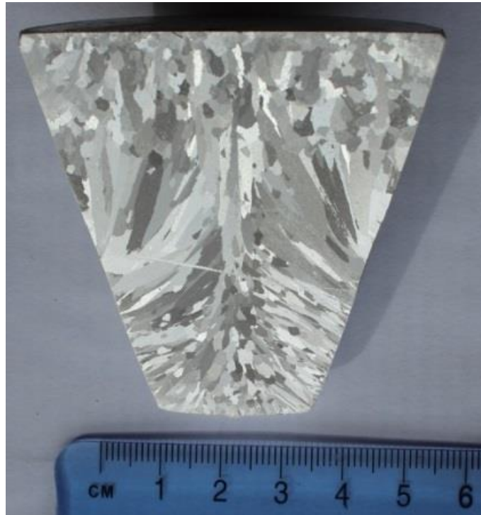
Fig 3.6 Macroetched vertical section of 0.8% Mg sample
