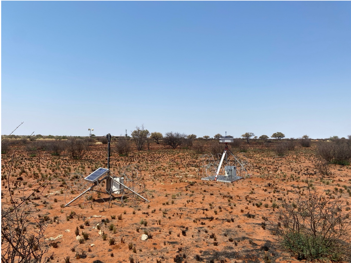
Figure 7.2. In-situ measurements of dust using a DustTrak monitor and meteorological station at site K02 burned interdune plot in September 2022.
