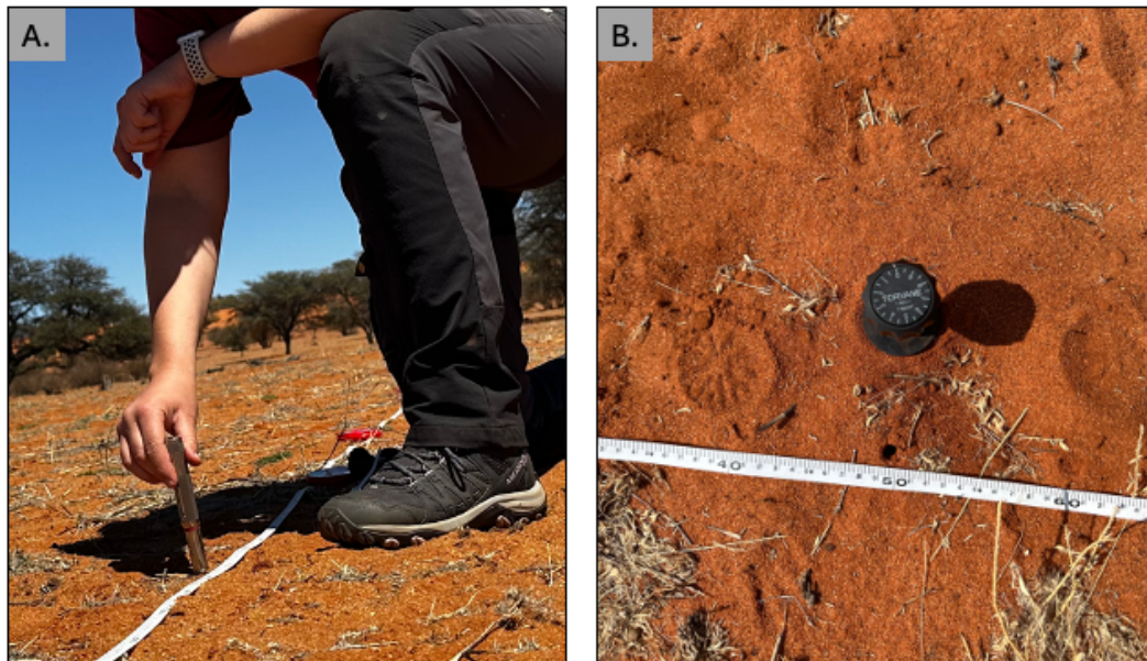
Figure 3.18. Measurements of surface properties recorded at 10 cm intervals along the 10 m transect at each field plot. (A) surface strength measured using a pocket penetrometer and (B) surface strength using a Torvane pocket shear vane.
