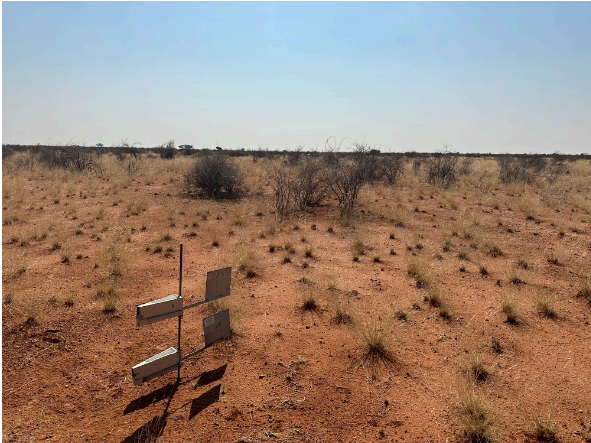
Figure 3.16. In-situ measurements of dust using two BSNE traps at site K02 burned interdune in September 2023 – 12 months after burning.
