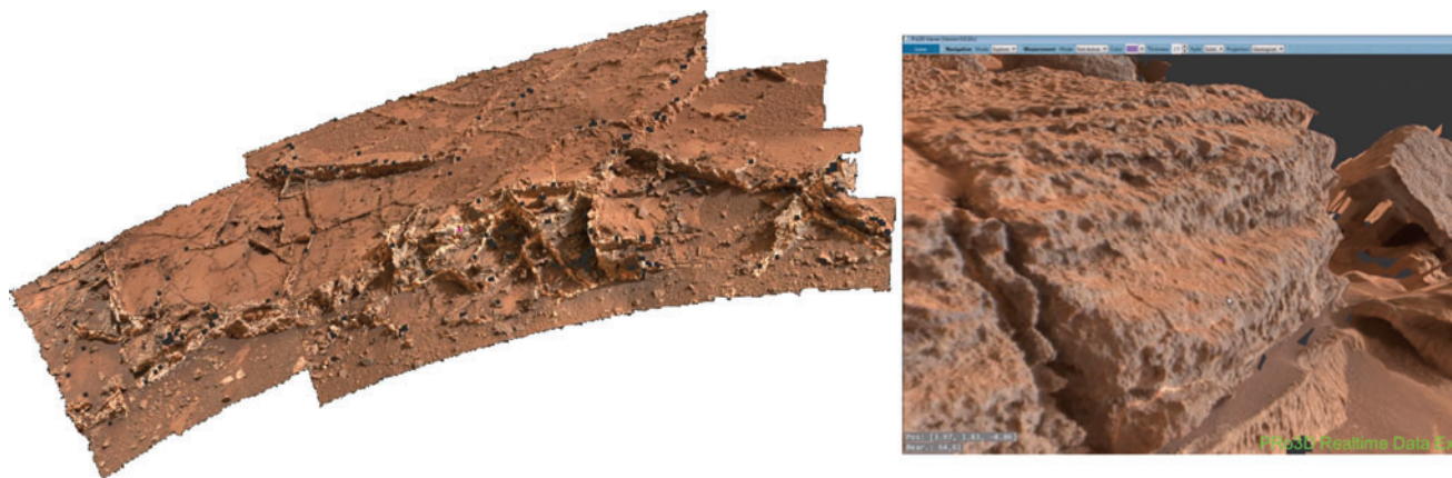
FIG. 14. (Left) Result of MSL Mastcam processing of Garden City outcrop area taken at MSL Sol 926 and 929 (DTM, rendered by PRo3D) making use of ExoMars PanCam 3-D vision processing workflow scheme PRoViP. (Right) 3-D rendered MSL Mastcam stereo processing results at subcentimeter resolution, as appearing in PRo3D Graphical User Interface.
