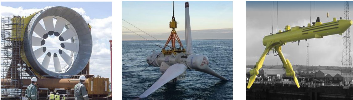
Fig. 1. 1 Examples of axial-flow tidal turbines. Left: Cape Sharp Tidal from OpenHydro Group Ltd. (2017); middle: AR1500 from SIMEC Atlantis Energy (2017); right: SR2000 from Orbital Marine Power Ltd (2020).
