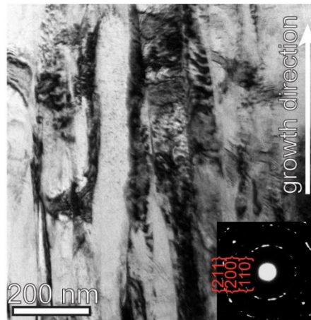
Supplementary Figure 3. Structure of the TiZrNbHf base alloy. Typical side-view transmission electron microscope (TEM) image, showing ~100 nm diameter columnar grains. The inset is the corresponding selected-area electron diffraction (SAED) pattern.
