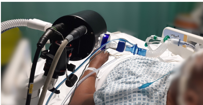
Figure 5.1: Photograph of the MFS measurement head connected to a mechanically ventilated participant in the ICU. The ETT is connected to the MFS measurement head via a catheter mount, end-tidal CO_2 sensor, and HME filter. Both the inspiratory and expiratory limbs of the ventilatory tubing connect to the non-participant end of the MFS head. The MFS head is supported by an adjustable arm; the adjustable arm in turn is connected to a pole attached to the hospital bed (not in picture). Photo courtesy of Dr Jessica Luiz, Department of Physiology, Anatomy and Genetics, University of Oxford.
