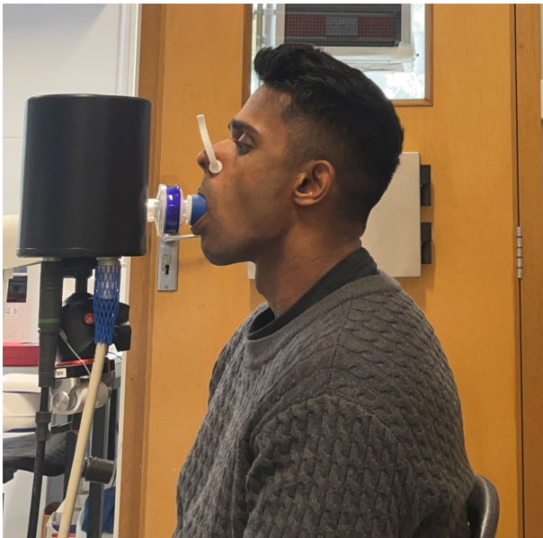
Figure 2.5: Picture of a volunteer wearing a nose clip breathing through the MFS measurement head via a mouthpiece and heat and moisture exchanger (HME) filter.
