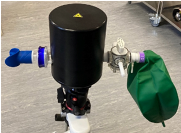
Figure 3.1: Picture of the reservoir bag attached, via a three-way tap, to the MFS head. The bag is attached to the opposite end of the participant end of the MFS head. The participant breathes through the MFS via a mouthpiece and heat and moisture exchanger (HME) filter. During the air-breathing phase, the three-way tap is open to the participant end and air; during the rebreathing phase, the tap is turned to allow the participant to respire into the bag.
