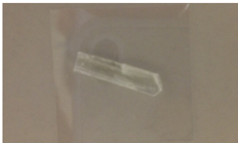
Figure 5.8: Anthracene single crystal grown by an evaporation technique. The crystal was 14 mm in length and 4 mm wide.
