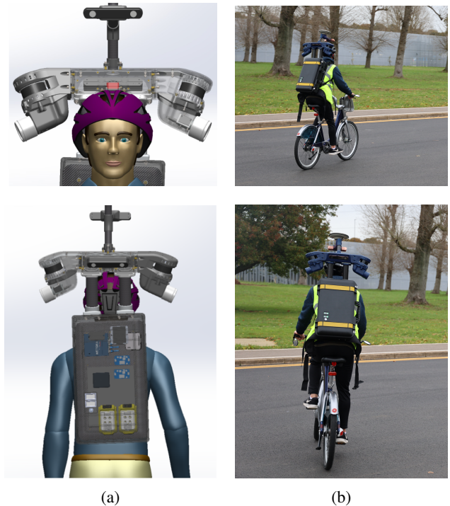
Fig. 1: Data-collection platform design (a) and deployment (b). The sensors and computing unit have been integrated into a backpack, allowing application flexibility without compromising the specifications and FOVs of the sensors.
