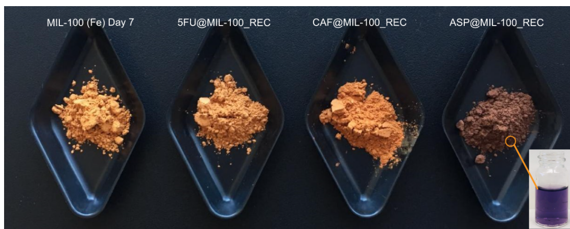
Figure 6.21: Photograph showing the various MIL-100 (Fe) samples after the encapsulation reconstruction process, showing a distinct colour difference between 5-FU@MIL-100_REC and CAF@MIL-100_REC to ASP@MIL-100_REC. This is due to the formation of a violet aspirin-iron complex known as tetraaquosalicylatroiron (III) complex (inset). When in contact with moisture, aspirin dissociates into acetic and salicylic acid. The latter then can react with acidified iron (III) ions to form the violet complex.
