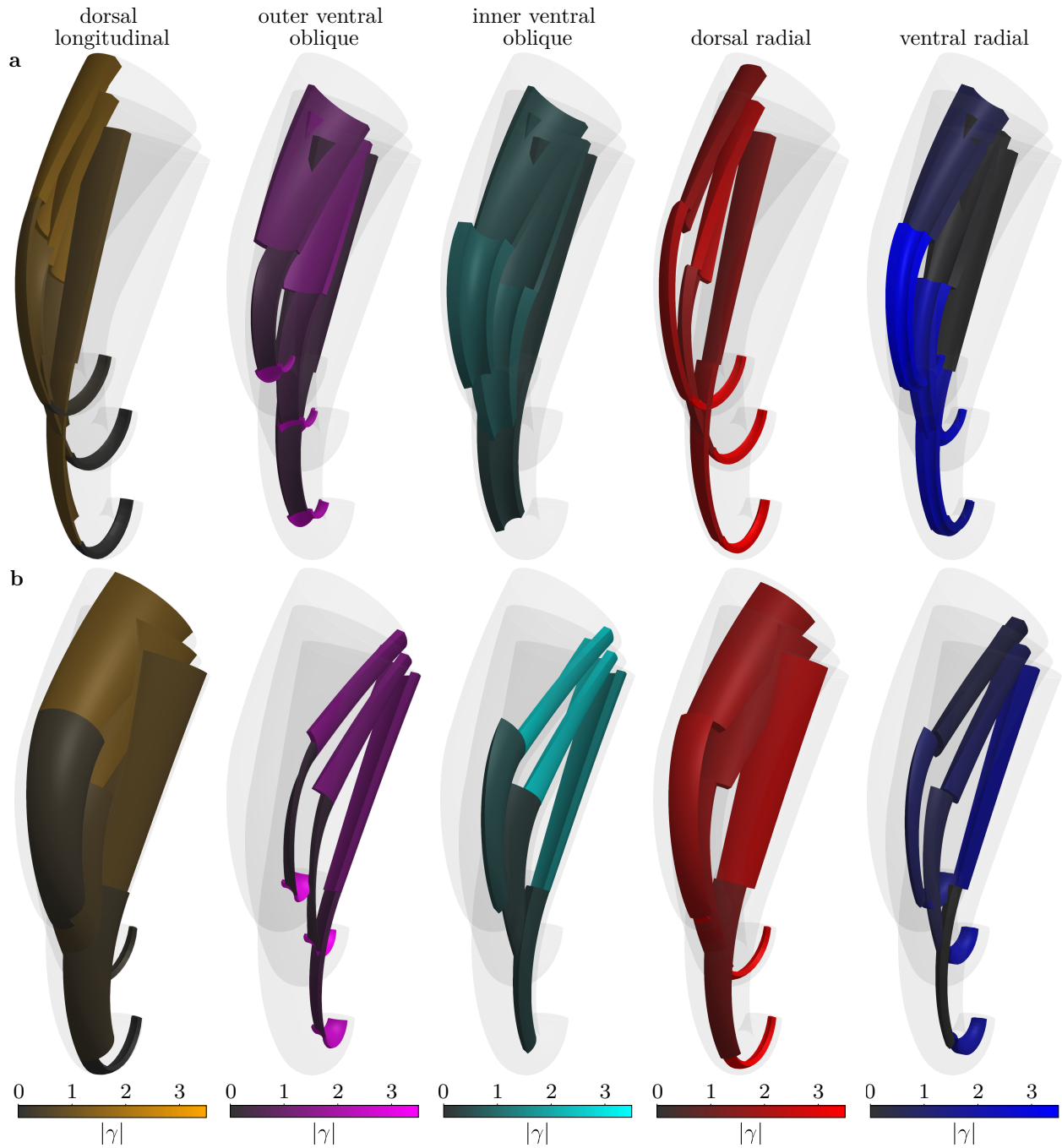
Figure 7: Isolated views of the individual muscle groups and their activations during the log lifting task. We color-code the muscular subdomains according to their corresponding activation magnitudes at three time points in the (a) right and (b) left trunk during the third motion phase. Each column corresponds to one muscle group associated with one color bar legend.
