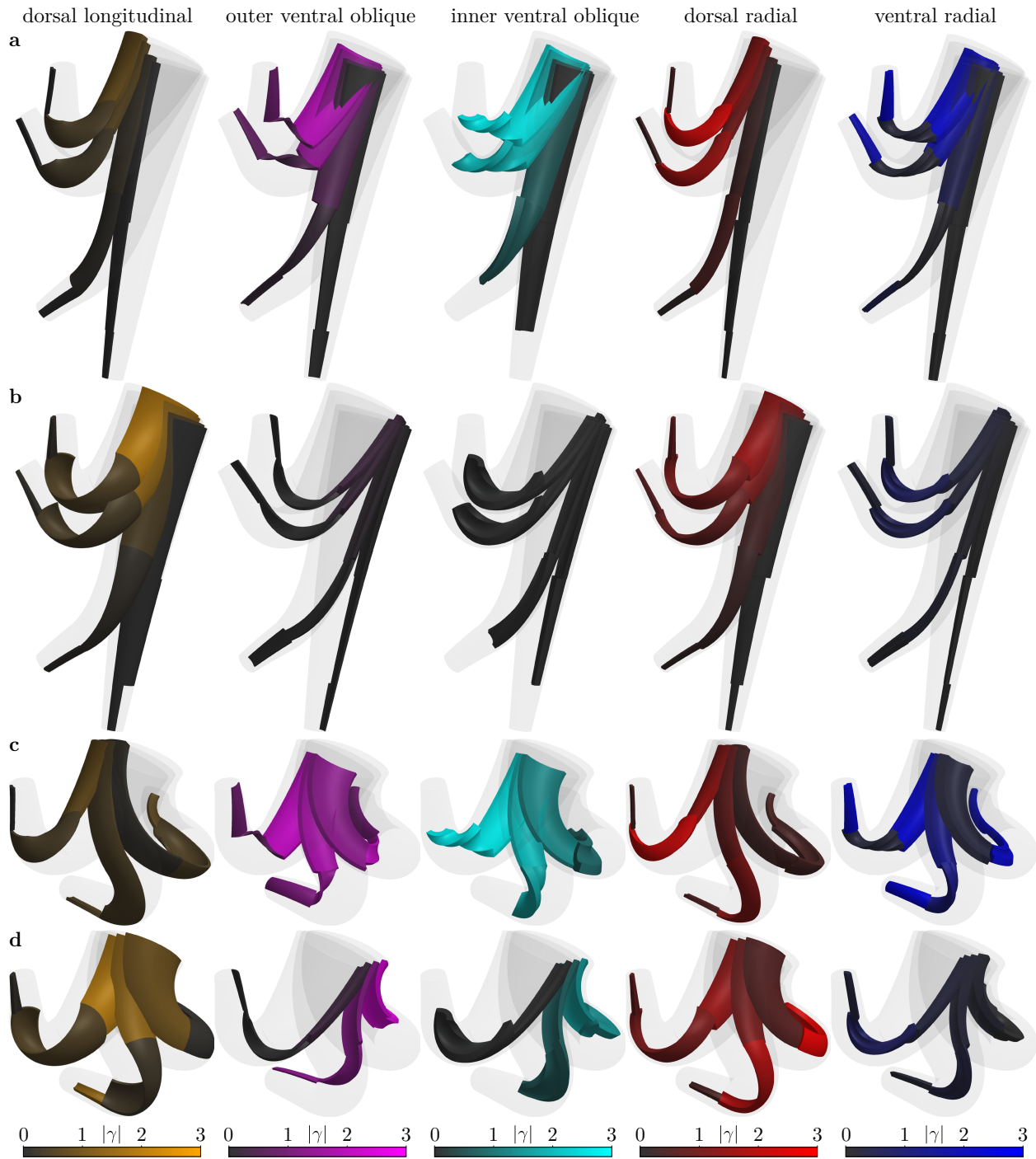
Figure 5: Isolated views of the individual muscle groups during the fruit-picking motion. We color-code the muscular subdomains according to their corresponding activation magnitudes at multiple time points in the (a) right trunk during the first motion phase, (b) left trunk during the first motion phase, (c) right trunk during the third motion phase, and (d) left trunk during the third motion phase. We show four and three consecutive deformations in the first and third phases, respectively. Each column corresponds to one muscle group associated with one color bar legend.
