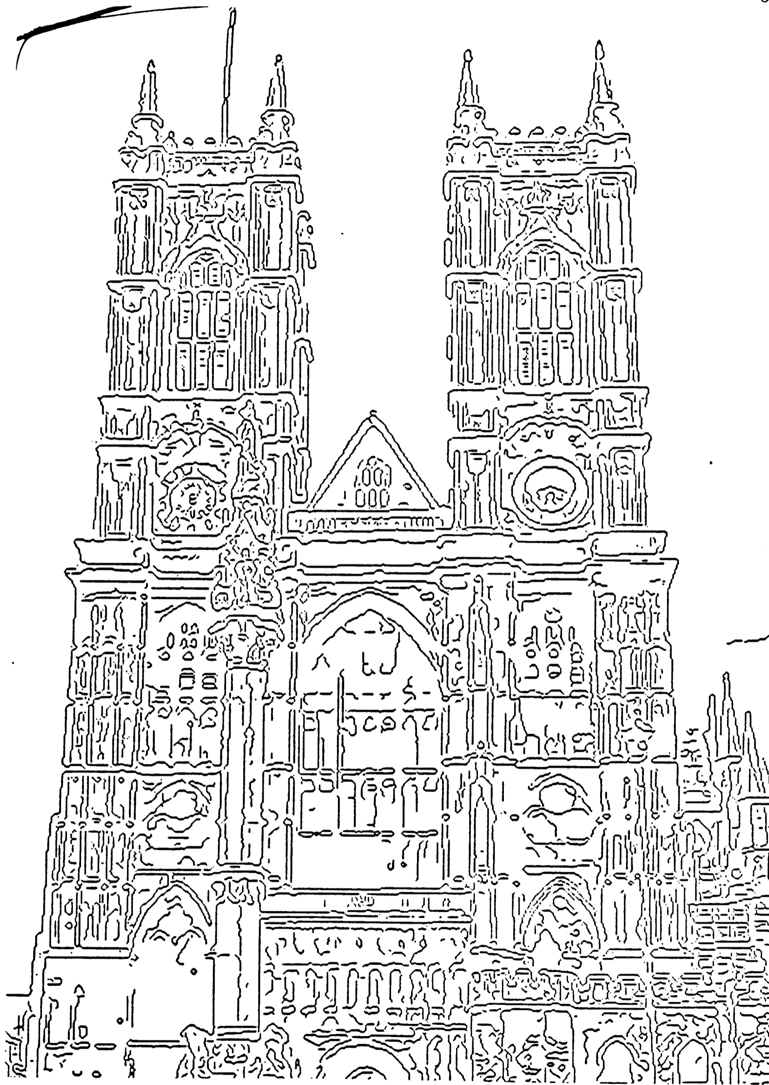
Figure 2.10: Showing the results of the application of Canny's edge finder to the Westminster Abbey image. Note the good performance of the algorithm over areas of varying contrast.
