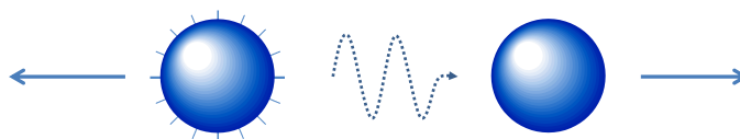
Figure 1.21 Recoil of a nucleus upon absorption or emission of a \gamma -ray.
