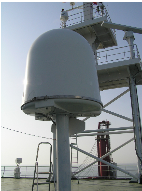
Figure 5.1: A typical marine VSAT system [156].
