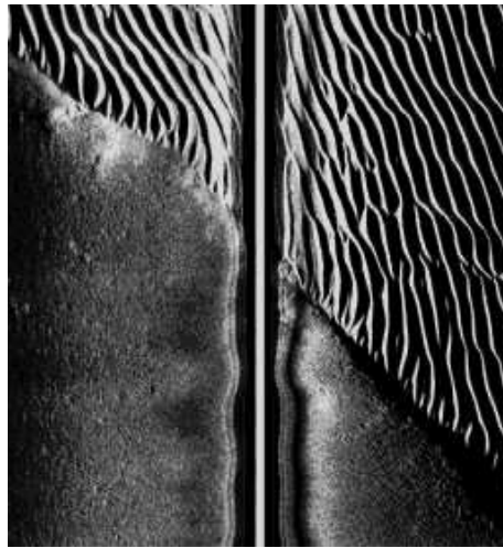
Figure 11.1: Sand Ripple sidescan image obtained by a very high resolution sonar at 900 kHz, by Marine sonic ( http://www.marinesonic.com/archives.html ). The sonar we used (234 kHz) was of a much lower resolution, and sand waves were not that evident.
