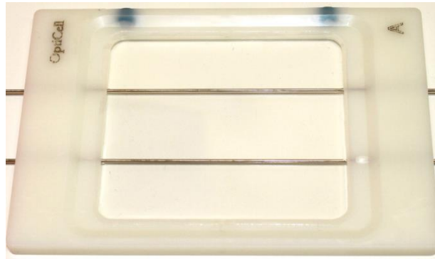
Figure 4.1: Opticell mould model used to create the tumour tissue-mimicking phantom. Two 1-mm stainless steel bars are used to create flow-channels in the phantom after agar embedded with cancer cells were injected into the mould.
