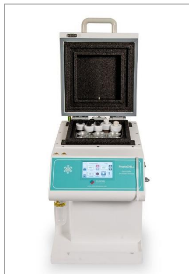
Figure 2.1 Image of PrestoCHILL instrument. The tissue sample is placed onto aluminium molds for rapid freezing (approximately 60 seconds). The instrument features a touch screen interface for setting tissue processing parameters.
