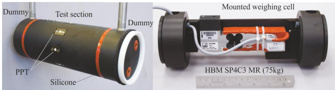
Figure 3-4 Model pipe used in the testing rig (Source: Schupp, 2009). The internal load cell measures the resultant of the external soil forces acting on the central test section.
