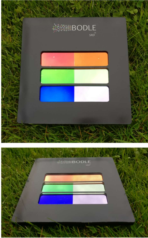
Figure 2 – RGB static samples in the vivid (left) and pale (right) states at two different angles on a cloudy afternoon. No contrast enhancement of any kind has been applied to these pictures.
