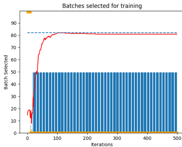
Figure 6.9: The teacher data selection as well as the performance of the student on the held-out test set for the MNIST digit recognition problem. The orange 'x' and blue bars represent the first and second outputs of the teacher respectively. The dashed line shows the maximum accuracy achieved. The red line is the performance of the student on the held-out test set.
