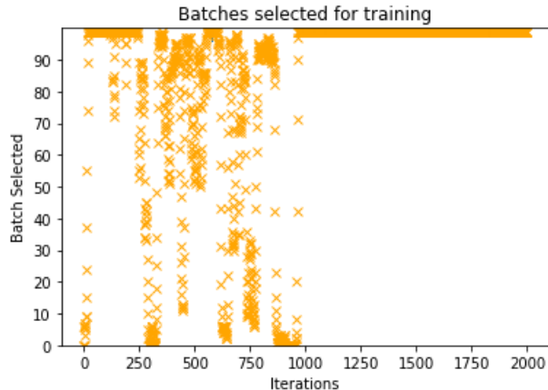
Figure 5.14: Actions generated by the policy of a constrained DDPG teacher on the CIFAR-10 dataset where it is highly probable that only one datapoint will be selected at a time for training. We see that the selection is significantly more chaotic. Batch numbers near zero are low entropy data and batch number 100 contains the highest entropy data.
