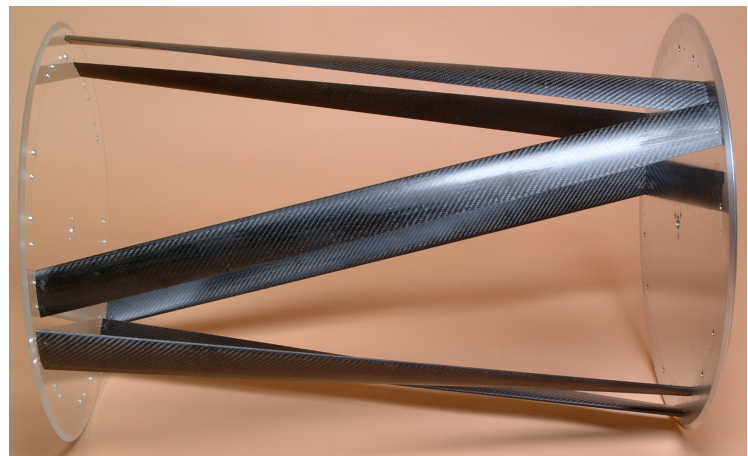
(b) Transverse Horizontal Axis Water Turbine (THAWT)
