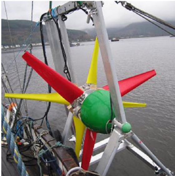
(a) Contra-rotating marine turbine, taken from Clarke et al. (2008)
