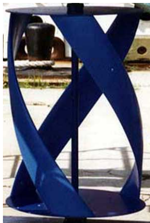
(a) Gorlov turbine, taken from GCK Technology (2011)
