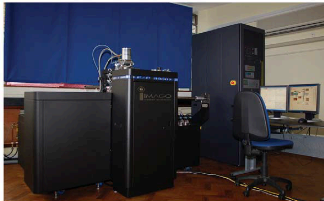
Figure 2.8(a) Schematic representation of a 3D local electrode atom probe. The atoms are field evaporated from the apex of a needle-shaped specimen by application of a high electric field between the counter (local) electrode and the specimen (as shown inset). (b) View of the LEAP™ 3000XSi in Oxford. Reproduced from reference. [14][13]
